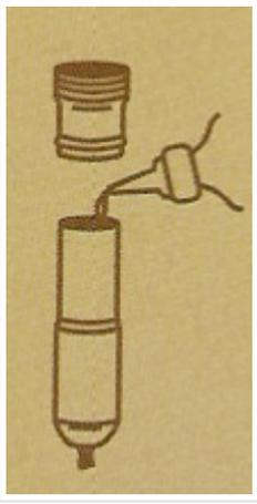
Pull the fuel chamber downward, out of its casing. Hold with wick side down and pull the cap off. Slowly fill the cotton-filled fuel chamber with fluid until approximately three drops of fluid fall from the wick. Replace the cap and return the fuel chamber to its casing.
