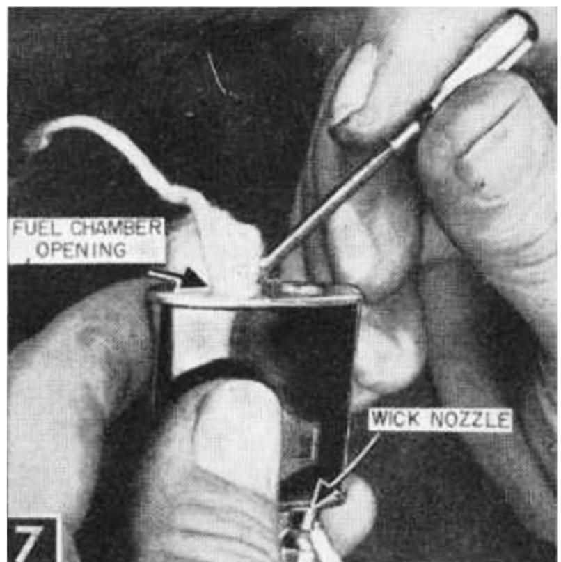
Stuff small wads of absorbent cotton through fuel chamber opening, alternating from side to side of case, until half of lighter is solidly packed. Push lower end of wick back into lighter; fill rest of lighter with cotton. Push all but about 1/16 in. of other end of wick down through nozzle.
