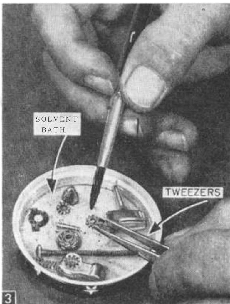
Immerse all working parts in cleaning solvent, such as lighter fluid. Scrub each part with a small brush dipped in solvent and set aside on clean paper to dry. Remove all wadding in fuel chamber and pull wick out through nozzle.
