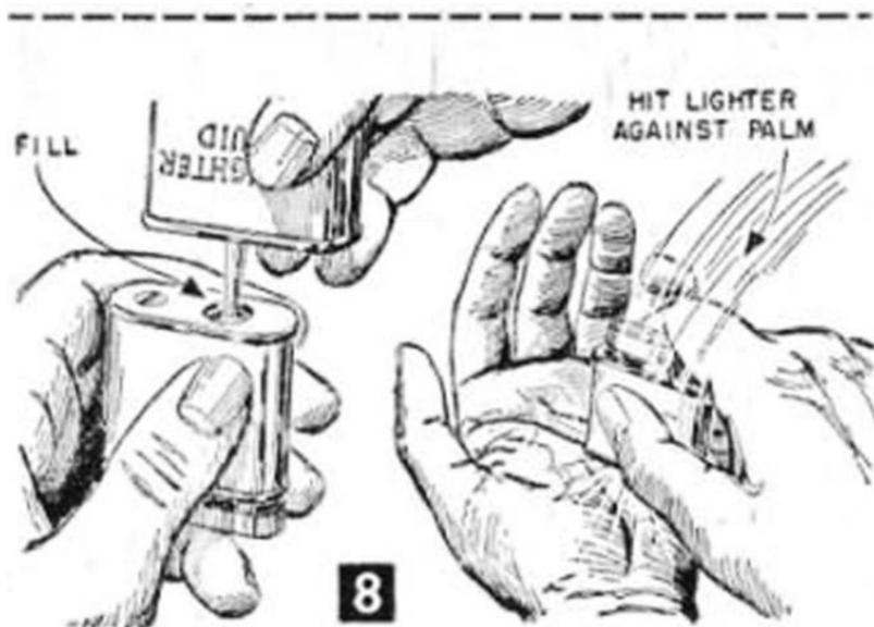
When wick is entirely surrounded by cotton so all sections will be continually saturated by fuel, fill lighter with fluid through fuel chamber opening until cotton will absorb no more. Hit lighter, opening down, sharply against palm of hand to remove excess fluid, then screw in cap tightly.
