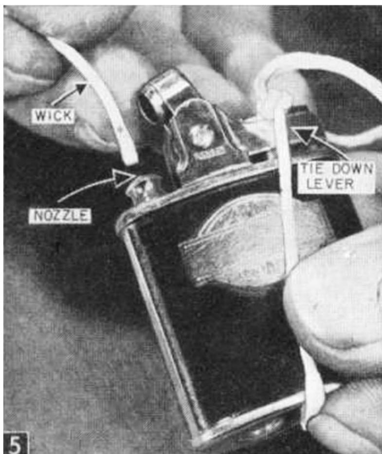
Reassemble lighter except for two bottom caps, tie down wheel lever and insert new wick in nozzle. Roll end of wick between thumb and forefinger or coat with nail polish to make an insertion point
