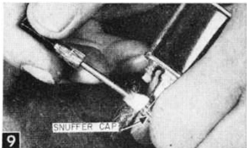
Wipe inside of snuffer cap with pipe cleaner or small screwdriver wound with cotton. Drop a new flint into flint cap opening, insert pressure spring and then screw in the flint cap.
