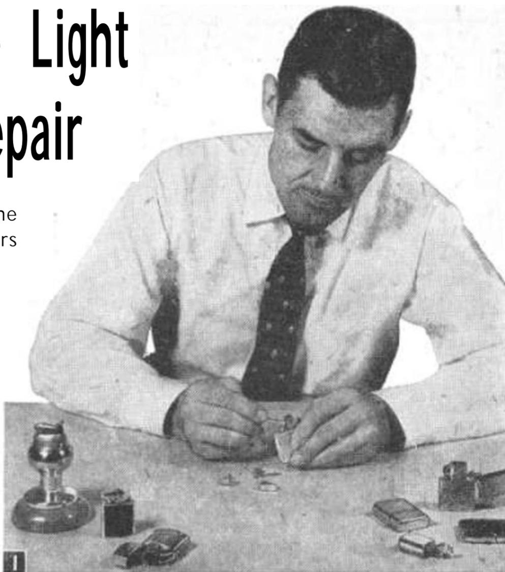
First step in overhauling a cigaret lighter is to take it completely apart. Use a small screwdriver for this job. Remove flint screw cap and pressure spring before taking off spark wheel, or flint may pop up in your face when no longer restrained by spark wheel.
